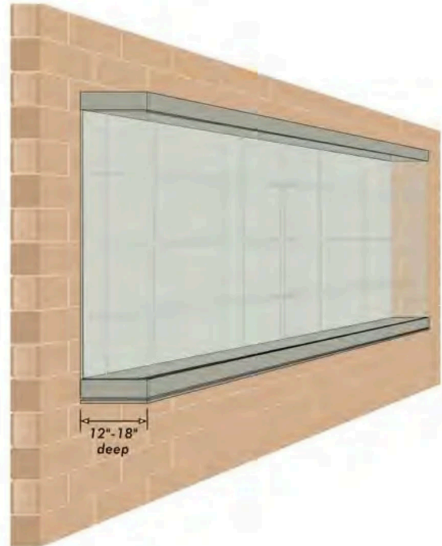
» lower section display case & wall mount detail
