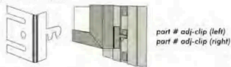
» marker board / tack board, clip, and mount detail
